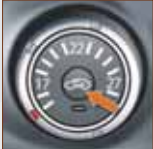
Exterior air intake. Interior air recirculation.
